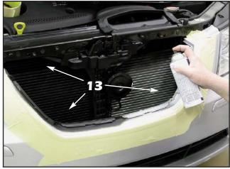
13. Apply flat or semigloss black paint to everything that will be visible through the E&G grille once it is installed. On vehicles painted colors other than dark blue or black, use a scotch brite pad to scuff the paint around the grille opening and paint the return edge of the grille opening inside the mounting pin holes as well.
