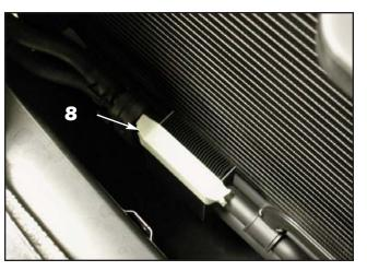
B. IMPORTANT: Use masking tape to cover the fins on the small cooler located on the passenger side near the bottom of the radiator. The fins are very sharp and you could easily cut yourself while installing the mounting hardware on the lower mesh grille.
