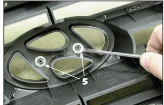
Remove the factory emblem from the grille by removing the push on retainers securing the emblem into the factory emblem recess. Insert a small flat blade screwdriver in between the retainer and the grille and twist to remove.
