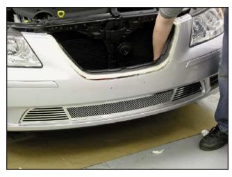
11. Install the lower grille section first, accessing the mount ing hardware from the top. The rectangular 3 hole mounting brackets install over the studs and the black plastic washers install on the remaining studs. Snug the hardware but do not overtighten as you will indent the lower grille frame where the studs are located.
