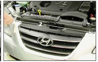
2. Remove the two (2) 10mm hex bolts from the bumper cover (one each side). Save for reinstallation.
