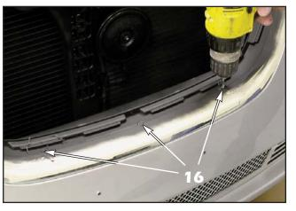
16. Use a .125" (1/8") drill bit to drill through the marks made in the previous step, then using the drill bit, connect the holes to form a small slot for left to right grille adjustment. Remove all plastic shavings from the bumper cover.
