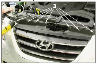
3. To remove the stock upper grille, you must first remove the seven (7) phillips screws across the top of the grille.
