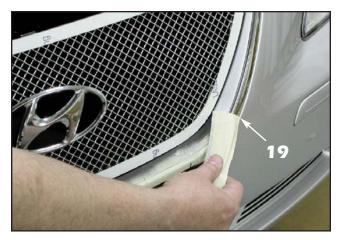
**19.** Carefully remove the protective masking tape from around the grille opening. The tape could get caught under the grille. If it does, lift up slightly on the grille while removing the tape.
